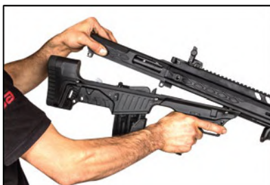
6) Separate the Upper Receiver from the Lower Receiver
