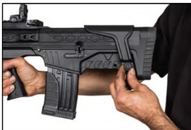
4) Take out the Cheek Piece Setting Plug and Cheek Piece Setting Plug Nut
