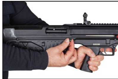
5) Pull the Upper Receiver Pivot Pins and handguard pivot pin to take out
