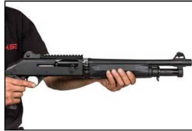
2) Slide The fore-end off the magazine tube
