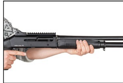
2) Slide The fore-end off the magazine tube
