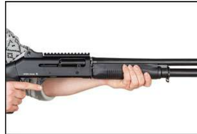
2) Slide The fore-end off the magazine tube
